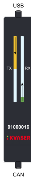
Figure 6: The TX LED bar lights up from the USB side to the CAN side of the unit, while the RX LED bar lights up from the CAN side to the USB side of the unit.
