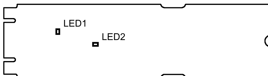
Figure 5: LEDs on the Kvaser M.2 PCIe 4xCAN.
